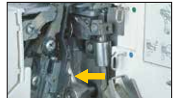
Easy to Remove Stitch Finger for Narrow/Rolled Edge
