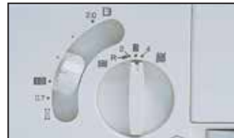
Outside Differential Feed Control
